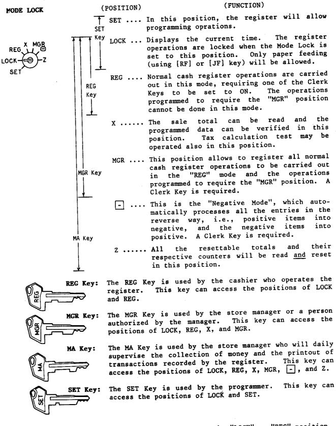
The keys may be inserted or pulled out at the "LOCK" or "REG" position.
